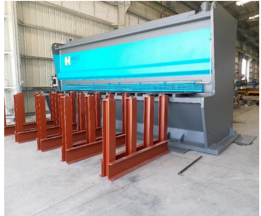
Name: CNC Shearing Machine Brand: HACO NV/HACO, Belgium Purpose: Shearing of Plate – 16 mm thk, 6 meter lo
