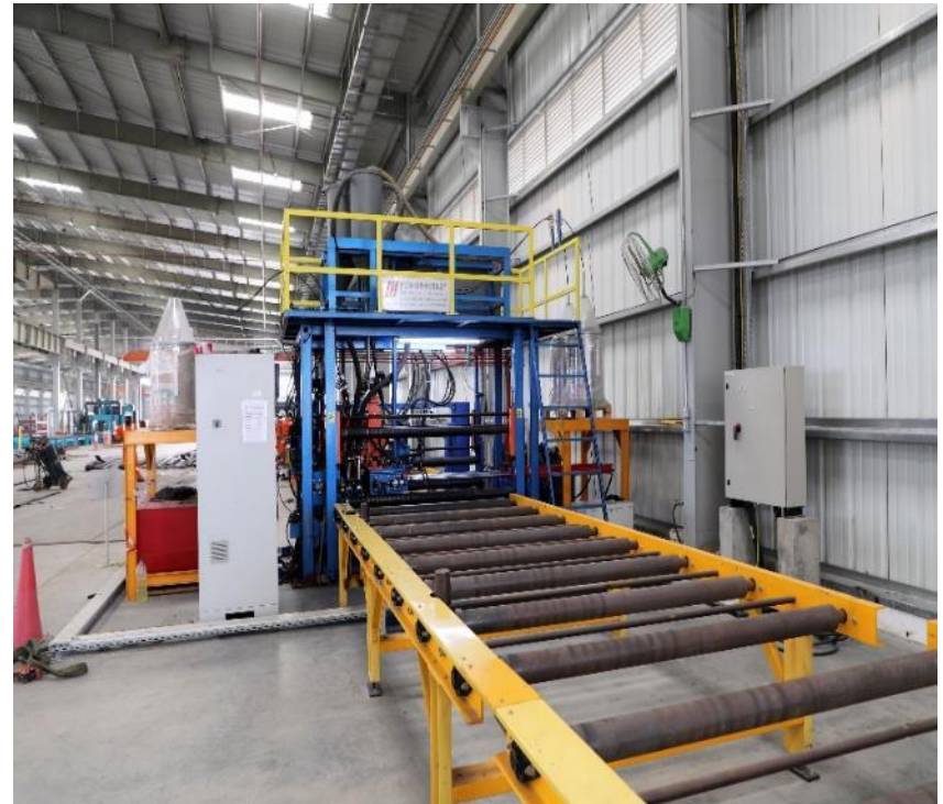
Name: H- Profile Welding Line Brand: Zhejiang Jinggong/JH-150A Purpose: Beam Welding Line
