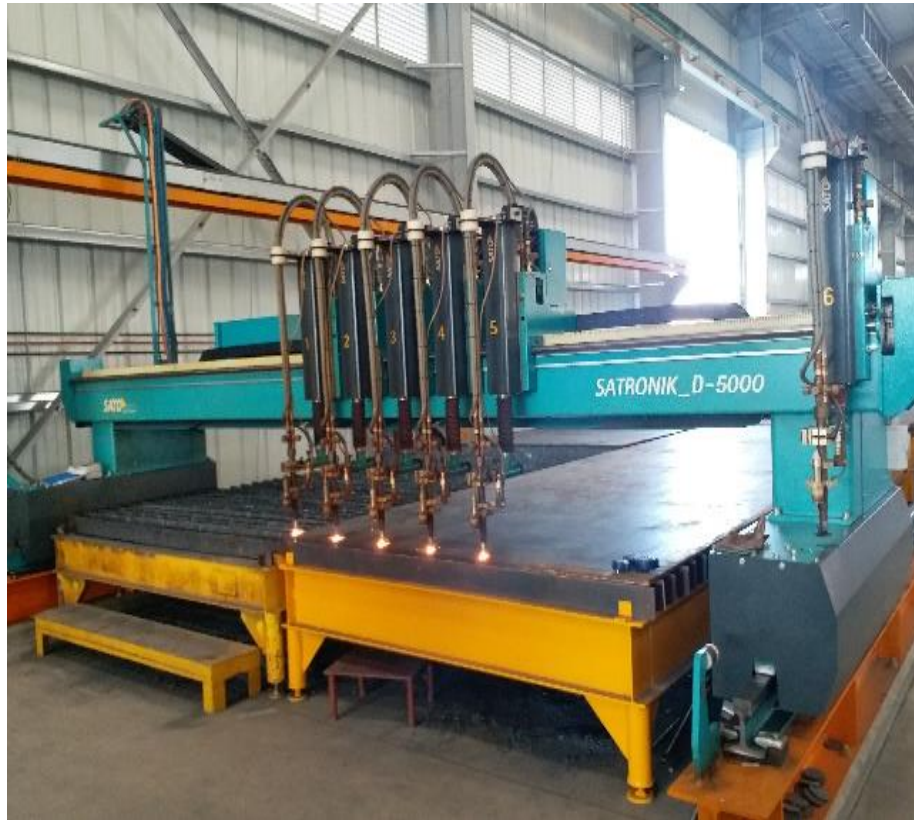
Name: CNC Cut & Strip Machine- 4.02 M x 12 M Brand: SATO/ Satronik D5000, Germany Purpose: Oxy-Acetylene Cutting of Plates & Strips
