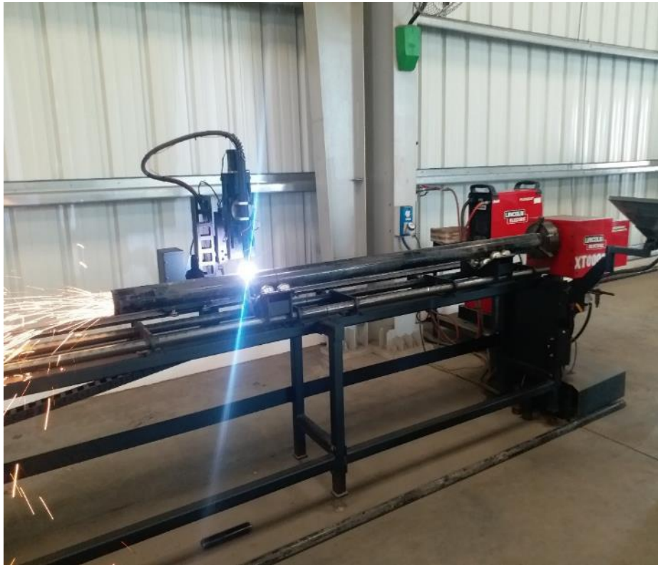
Name: Pipe Profiling Brand: Lincoln, USA Purpose: Pipe Profile Cutting
