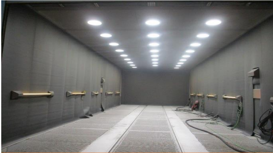
Name: Shot Blasting Chamber, Scitex, Poland
