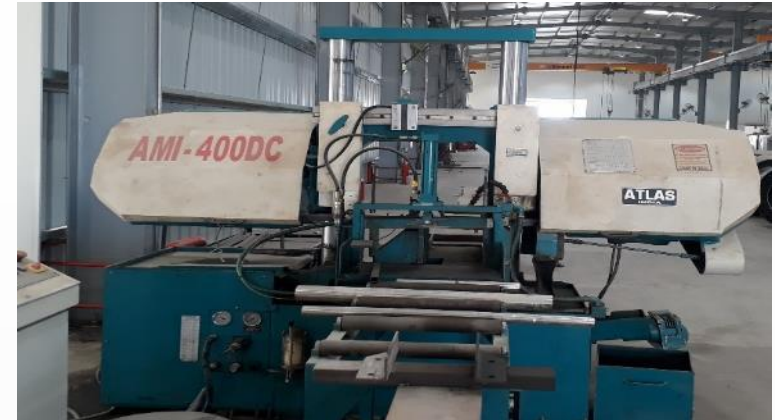
Semi automatic band saw for bar and pipe cutting
